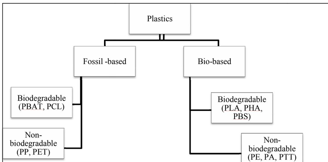
**Fig. 1. Classification of plastics based on their composition and degradation**
